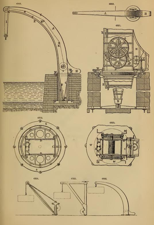
the next five, which have to resist the horizontal thrust against the cast-iron circle at the top edge of the well,  $\frac{3}{5}$  in. thick; and the remainder  $\frac{5}{16}$  in. thick. The front of the crane is constructed with four cells, to resist the great strain of compression
